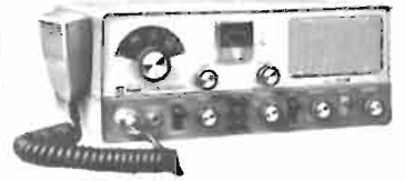
Knight-Kit® 6-Meter Amateur Transceiver with universal solid-state power supply.
