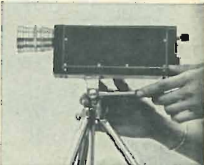
TINY TV CAMERA for space and military use is one of the miracles of integrated circuitry. This one weighs 27 ounces, uses a one-inch vidicon camera tube, and requires only four watts of power.
