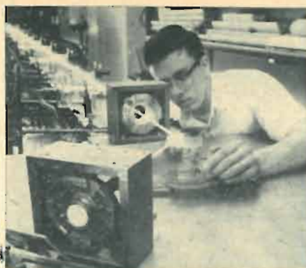
Laser beams for communications are able to be bent around corners by periscope devices. Here, a small prism is used as a passive relay device that changes the direction of the highly concentrated laser beam.
