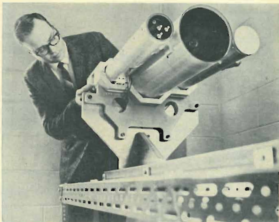
Sylvania engineer Robert Johnson inspects beam reflector (left tube), tracking telescope (center tube) and receiving unit (right tube) of the electrically scanned laser system.
