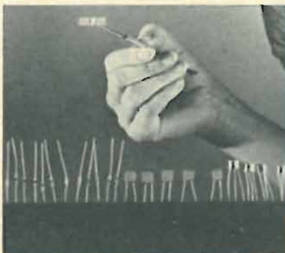
50 FUNCTIONS IN A SINGLE CHIP. The functions of these 50 separate transistors, diodes, resistors and capacitors can now be formed by the tiny dot in the center of the integrated circuit held by the tweezers.
